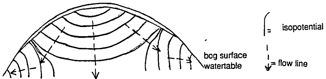
isopotentials and flow lines for a bog (and for a hummock- hypothesis) fig 1.
