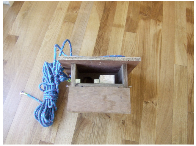
Figure 2: Weatherproof box used to protect the Anabat unit and 12V battery, front on left and rear (open hatch) on right. The image on the left shows the microphone hole. In the image on the right, the slot to hold the Anabat is visible on the left of the box and the slot to hold the battery is visible on the right.
