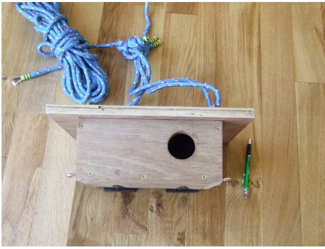
Figure 2: Weatherproof box used to protect the Anabat unit and 12V battery, front on left and rear (open hatch) on right. The image on the left shows the microphone hole. In the image on the right, the slot to hold the Anabat is visible on the left of the box and the slot to hold the battery is visible on the right.
