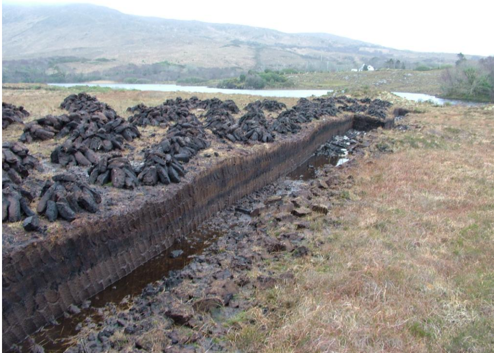
Plate 34: Cutting from a vertical surface, with vegetation re-establishment on the cut over area.
