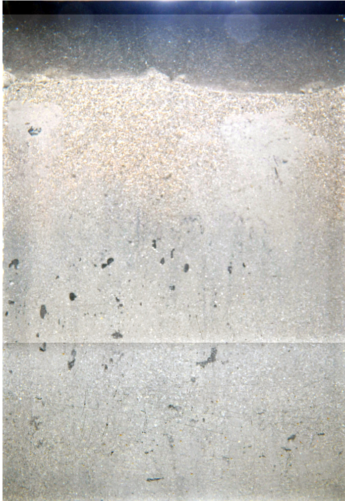
Sediment Profile Image of station 42 in the Barrow estuary showing mobile sand overlying recently deposited mud. The holes in the mud layer are not gas bubbles, they are water filled voids caused by violent deposition events, similar to spoil dumping. There appears to be an older, relict layer of mud at depth in the image. Image width is 13.7cm, penetration depth is approx 18cm.
