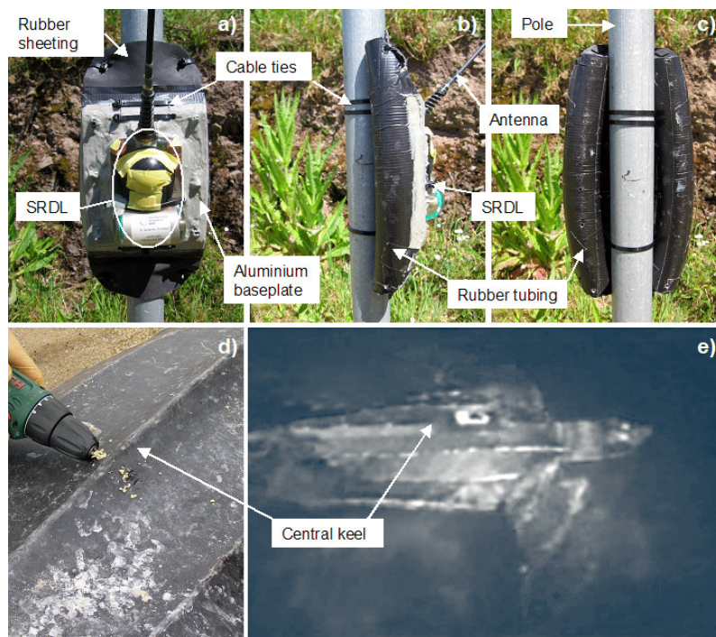
Figure 20: Illustration of direct attachment method. a-c) Top, side, and bottom view of SRDL/Baseplate attached to a vertical pole (60 mm diameter, and representing central keel of turtle) to demonstrate direct attachment method prior to deployment. Note cable ties run through baseplate and around the pole, with two at the anterior end and one at the posterior end. When cable ties are fully tightened the rubber tubing tightens around the pole (or keel) preventing any side-to-side movement of SRDL/Baseplate. Length of SRDL/Baseplate is 27 cm and weight (out of water) is 1 kg. d) Drilling 6.5 mm hole into right side of central keel of a leatherback turtle. Note drilling angle and that a similar hole was drilled into the central keel from the left side, with the two holes meeting in the middle. Cable ties are first fed through one hole in the baseplate, then through a hole in the keel,
