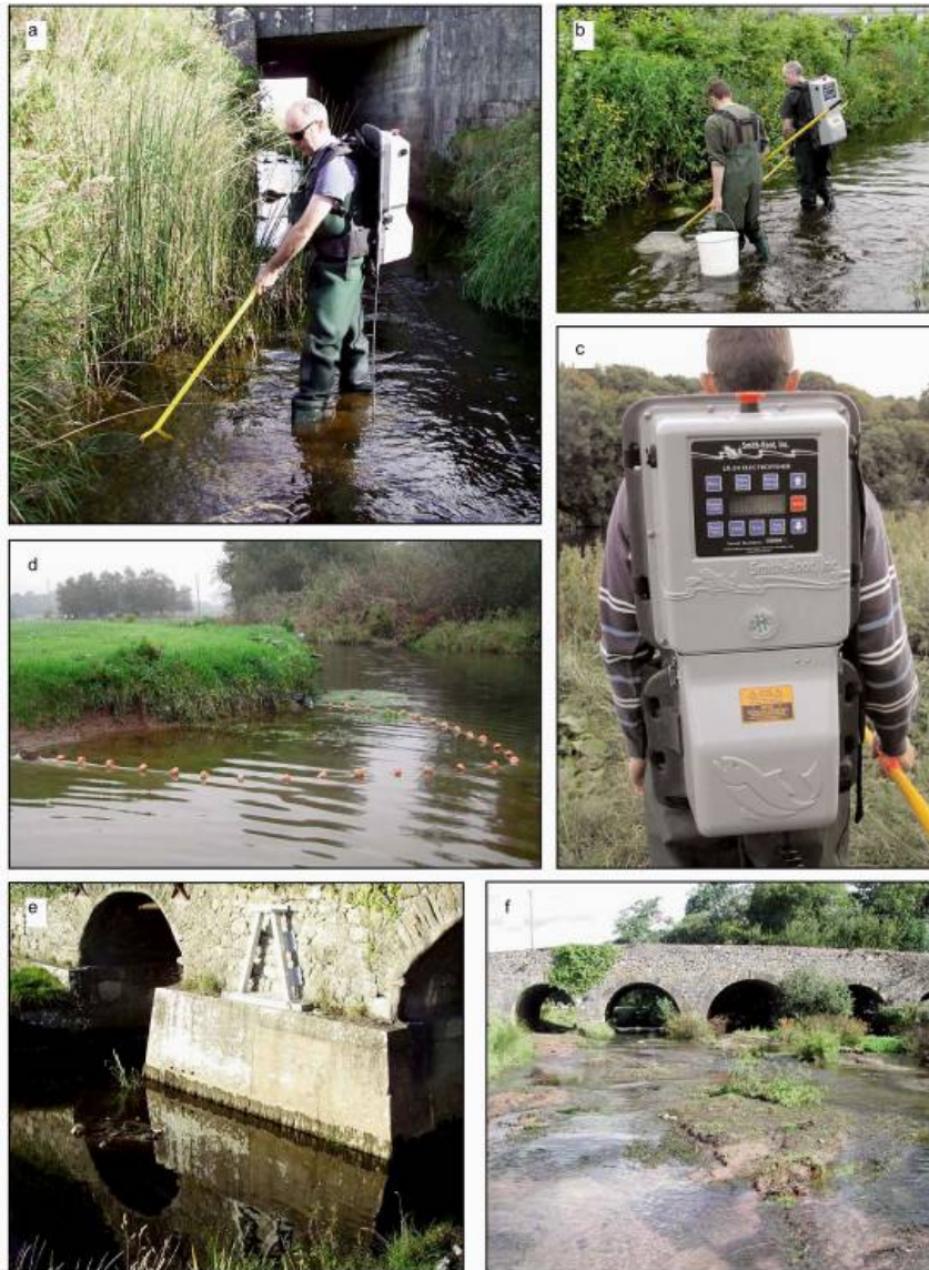
Plate 5 (a-f) (a, b, c) Electrical fishing with a Smith-Root LR-24 backpack electrical fishing unit, (d) quantitative electrical fishing survey on the River Suir at Ardfinnan, (e) survey section on the River Sinking – the site of the highest lamprey catch in the Corrib catchment, (f) the lower River Tar produced the highest lamprey catch in the Suir catchment.
