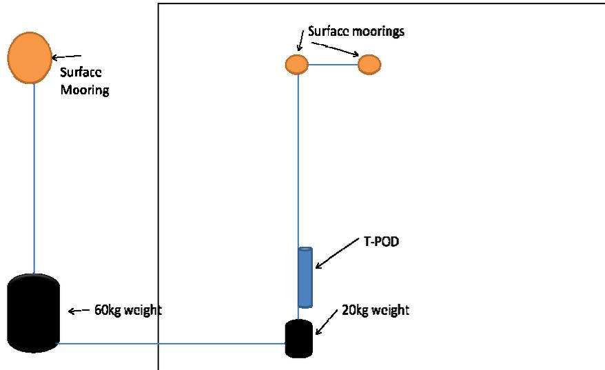
**Figure 3. Design of the mooring system used for deployment of T-PODs**
