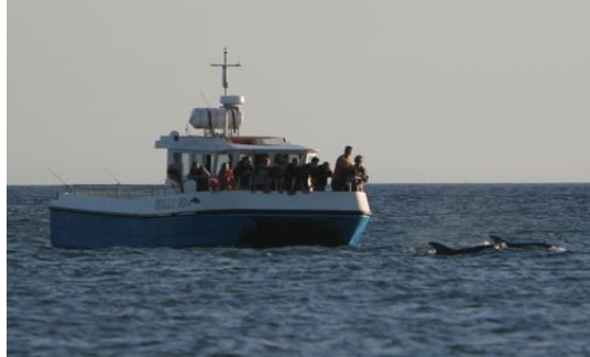
Figure 2. MV Holly-Jo with flying bridge suitable for line-transect surveying.
