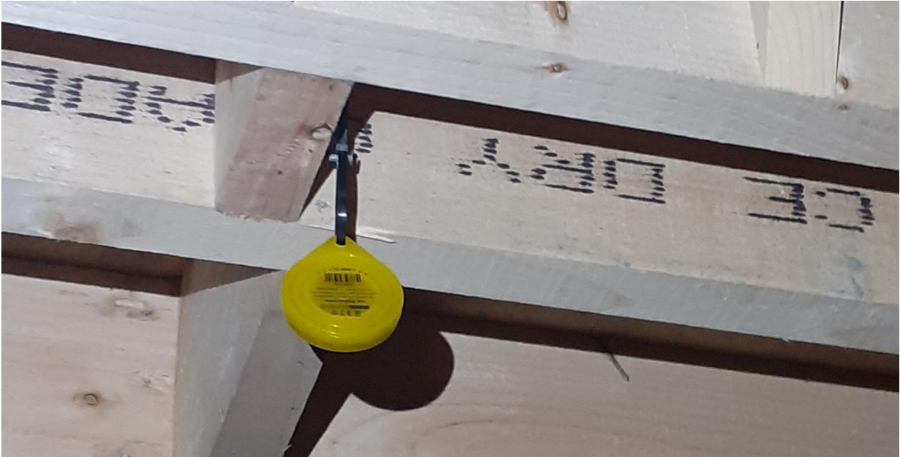
Plate 2: Temperature data logger installed in Bat House.
