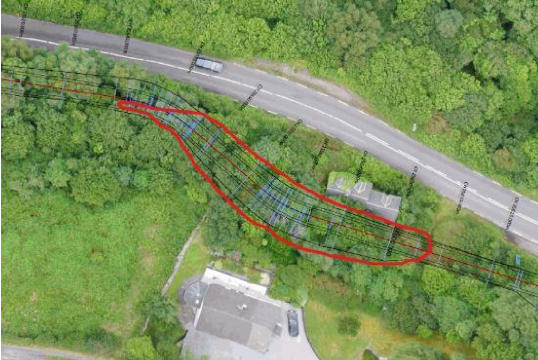
Figure 6: Extent of rock breaking works in vicinity of cottage is located in Red Line drawing.
