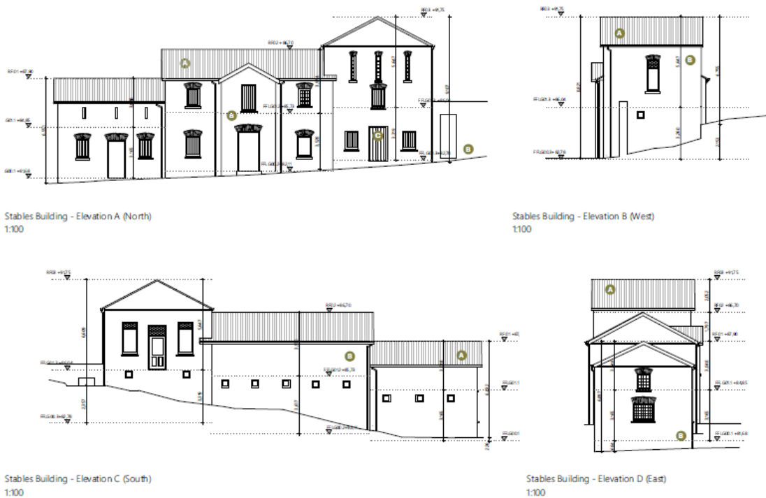
STABLES BUILDING & STORE BUILDING - EXISTING ELEVATIONS
