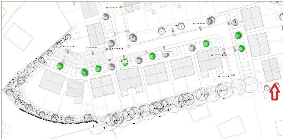
Figure 5.1 Proposed location of artificial bat roosts (indicated by red arrow) on southern gable of unit number 54.
