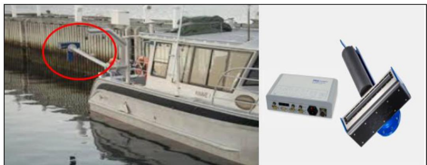
Figure 2.4 MBES R2Sonic 2024 typical configuration and equipment IMO 915882)
